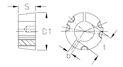
b = 22 Bore = 80 Bush type = 4040 D1 = 146 S = 101,6 Screw size =  $5/8 \times 13/4$ "
